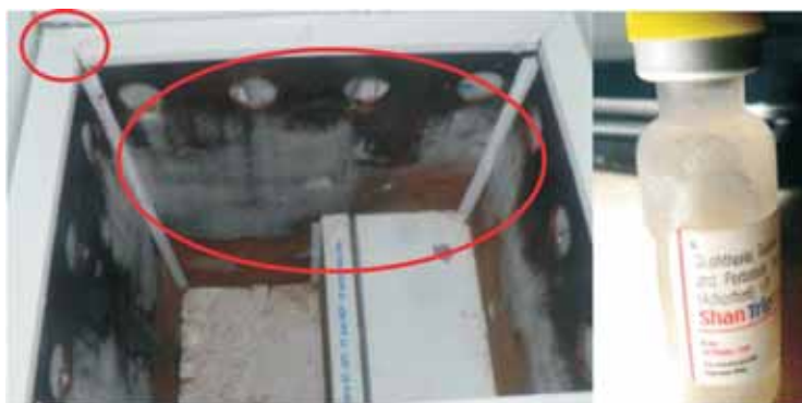
Old CFC ILR with frost and ice and froze in DPT vaccine
