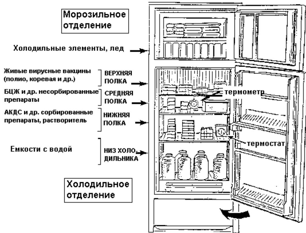
Figure 14: Loading a household refrigerator (Russian version)
