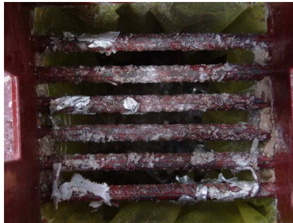
^ Aluminium caps caught on narrow spaced grill
