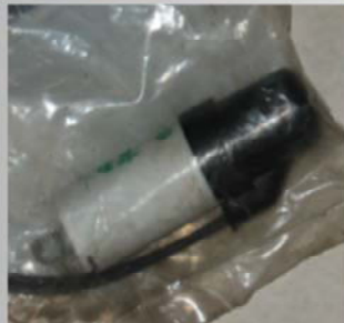
Capacitor condenser fan motor Code :0112 FOSTER cold room
