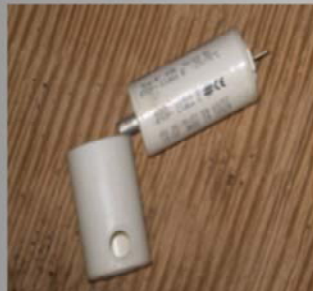
Capacitor fan motor: Code 0361 FOSTER cold room
