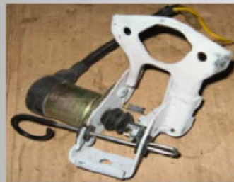
Stop solenoid: Code 0445 Diesel generator set
