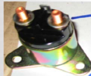
Starter solenoid: Code 0447 Diesel generator set
