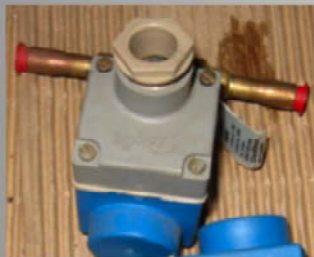
Solenoid valve: Code 0178 Diesel generator set
